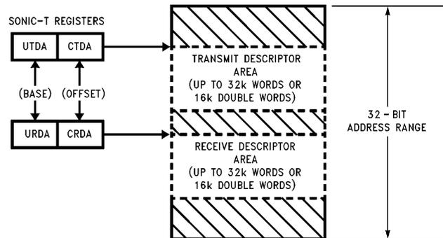
FIGURE 5-2. Transmit and Receive Descriptor Area Pointers
