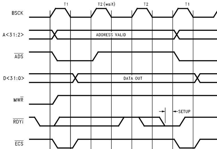
FIGURE 7-13. Memory Write, BMODE = 0, Synchronous (1 Wait-State)
