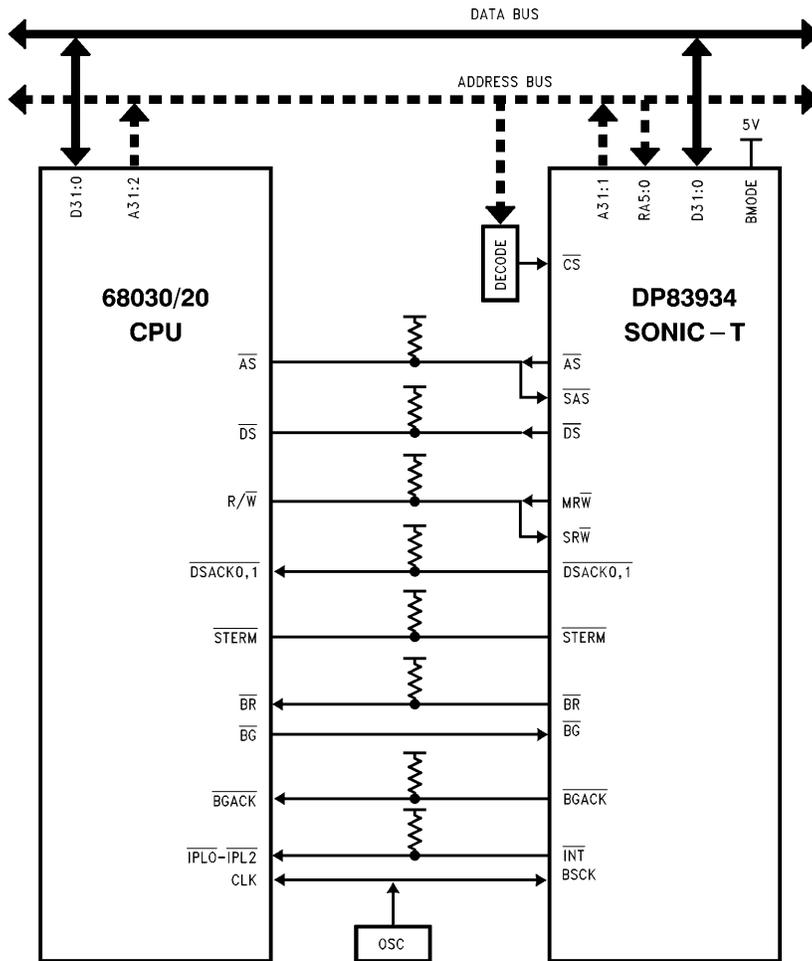
FIGURE 7-2. SONIC-T to Motorola 68030/20 Interface Example
