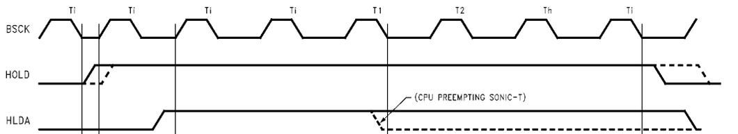
FIGURE 7-3. Bus Request Timing (BMODE = 0)
