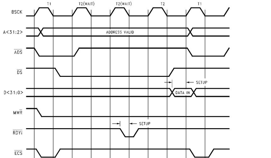
FIGURE 7-15. Memory Read, BMODE = 0, Asynchronous (2 Wait-State)
