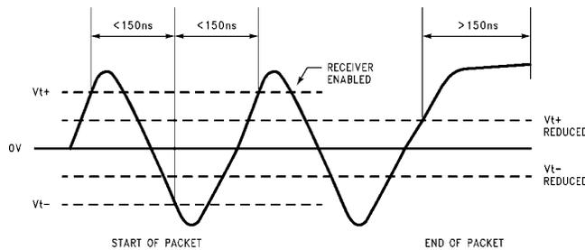
FIGURE 3-2. Twisted Pair Squelch Waveform (10BASE-T Mode)
