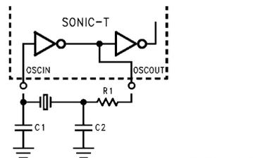
FIGURE 8-4. Crystal Connection to the SONIC-T (see text)
