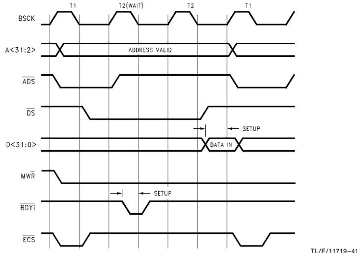
FIGURE 7-14. Memory Read, BMODE = 0, Asynchronous (1 Wait-State)
