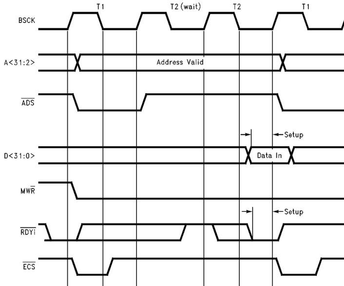
FIGURE 7-12. Memory Read, BMODE = 0, Synchronous (1 Wait-State)
