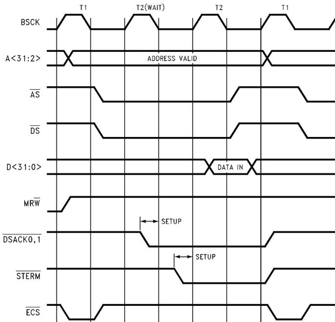
FIGURE 7-8. Memory Read, BMODE = 1, Asynchronous (1 Wait-State)
