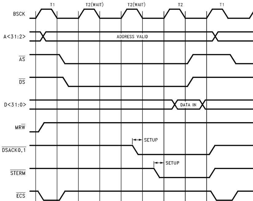
FIGURE 7-9. Memory Read, BMODE = 1, Asynchronous (2 Wait-State)
