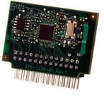
The CPM 5000 decreases product timeto-market for LONWORKS® based devices. It includes all the components needed to implement a control node using the FT 5000 Smart Transceiver — the smallest, fastest, highest performance, lowest cost twisted pair LONWORKS transceiver on the market.
