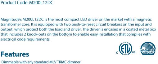
Dual protection - two manual push-to-reset circuit breakers on the primary and secondary sides Low operating temperature
