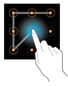
If you set a pattern lock, when the device disconnects from another mobile device, the pattern lock activates automatically.
