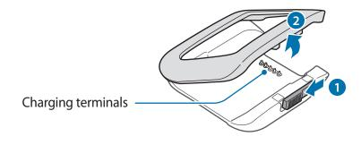
2 Place the device on the charging cradle with the charging terminals facing each other.
