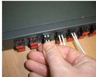
FIGURE 7 Push home to lock the clamp.
