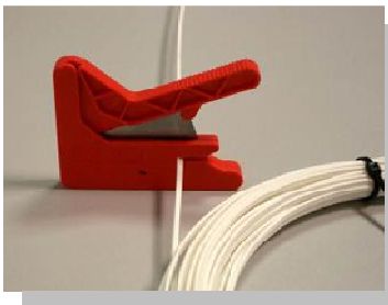
FIGURE 1 Cut the POF from its reel.
