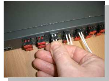
FIGURE 6 Insert and slide POF until it stops.
