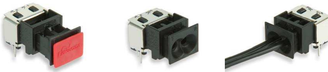
FIGURE 13: Side views of the OptoLock with dust cap, without dust cap and with POF inserted
