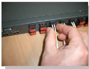
FIGURE 7 Push in the front clamp to lock POF into place.
