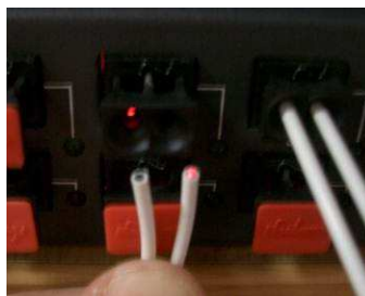
FIGURE 5 Present the lit core to the dark OptoLock side.
