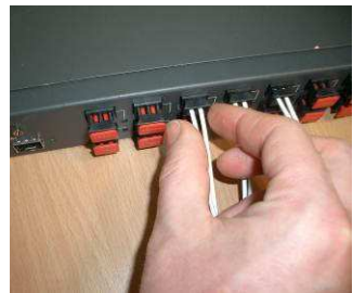
FIGURE 6 Insert both strands into OptoLock.
