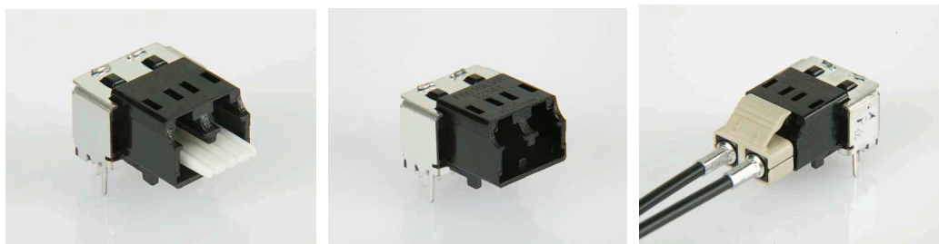
FIGURE 2 LC connector shown with dust plug, as open connector, and with LC plug inserted
