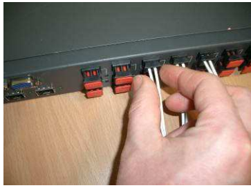
FIGURE 7 Push home to lock the clamp.
