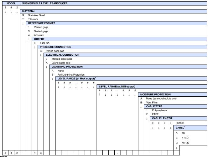
The part number requires two level range limits, corresponding to the maximum and minimum analog outputs of the transducer, to be specified in pounds per square inch (psi) to three decimal places. The lower level range is typically 000.000 unless otherwise required. For reverse output requirements, enter the lower level range for the maximum output signal and the upper range for the minimum output. Use the following conversion factors:
