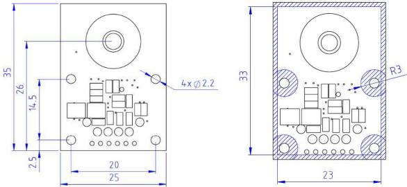
Only use hatched areas for mechanical assembly (screws, nuts, etc).
