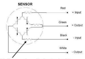
EPL-B0 compensation resistors in external module
