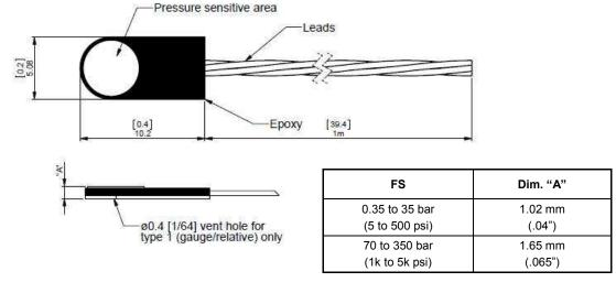
Note: EPL-D1 is internally compensated (no external module)
