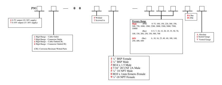
Examples: P90610002-7K5PSS = 0 to 5V output from 10 to 36V supply, cable outlet, welded 1/4" BSP male port, 7500 psi sealed gauge
