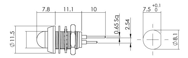
Dimensions in mm (typical) Not to scale Anode termination denoted by red indicator Mounting hole to be clean and burr free
