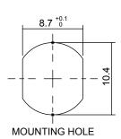
Anode termination indicated by long pin. Mounting hole to be clean and burr free.
