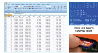
Transfer data from meter to PC using  $\mathsf{Excel}^{\otimes}$  software and datalogged readings from the SD memory card (included)
