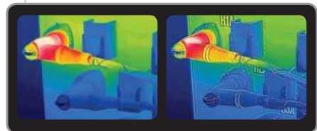
Original IR Image on the Left and with MSX™ Enhancement on the Right image (available on T640 model)
