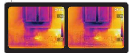
Original IR Image on the Left and with MSX™ Enhancement on the Right image (available on T440bx model)
