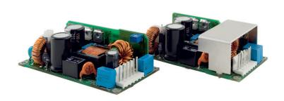
The new TOP-100 Series AC/DC Power Supplies feature the highest power rating in the industry standard  $2.0'' \times 4.0''$  ( $50.8 \times 101.6$  mm) footprint. They can supply up to 100 W output power with convection cooling over an industrial operating temperature range of  $-25^{\circ}$ C to  $+50^{\circ}$ C. This performance could be realized by a state of the art design providing an extremely high efficiency of >90 % which eliminates the need for a dedicated power supply cooling fan.
