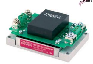
The TEP 200WIR Series is a family of isolated high performance dc-dc converter modules with ultra-wide 4:1 input voltage ranges. They come in chassis mount version with screw terminal block and with integrated EMI input filter to meet EN 55022 class A. A very high efficiency allows full power operation at 25°C with only 100 LFM air flow couling and operation at 60°C with only 40% power derating.
