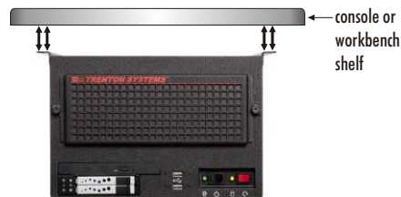
Front View - Upper mounting bracket position for mounting in a console or under a shelf
