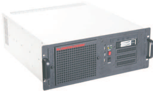
Trenton TRC4011 Rackmount System Shown with a BXT7059 SBC and a BPG7087 backplane
