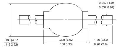
Note: The cathode side is marked with a dark colored band on one side of the diode body.
