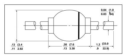
FIG. 306: Axial Lead Rectifier Outlines
