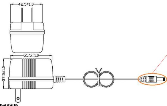
**Output Plug** and Polarity are **Dependent on** Customer Requirements
