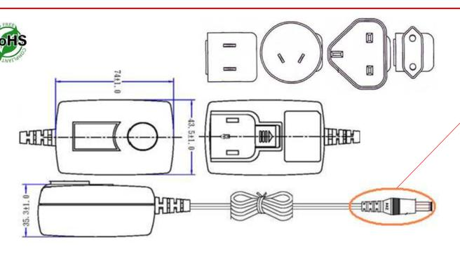
**Output Plug** and Polarity are **Dependent on** Customer Requirements
