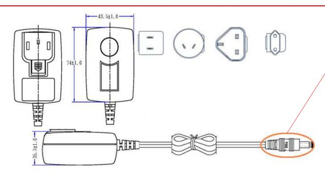
**Output Plug** and Polarity are **Dependent on** Customer Requirements
