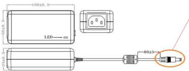
**Output Plug** and Polarity are **Dependent on** Customer Requirements
