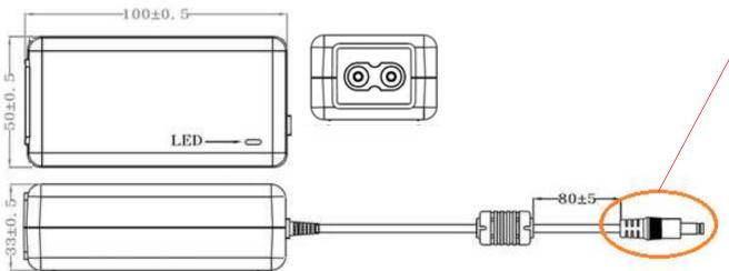
**Output Plug** and Polarity are **Dependent on** Customer **Requirements**
