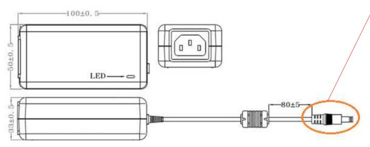
Output Plug and Polarity are Dependent on Customer Requirements
