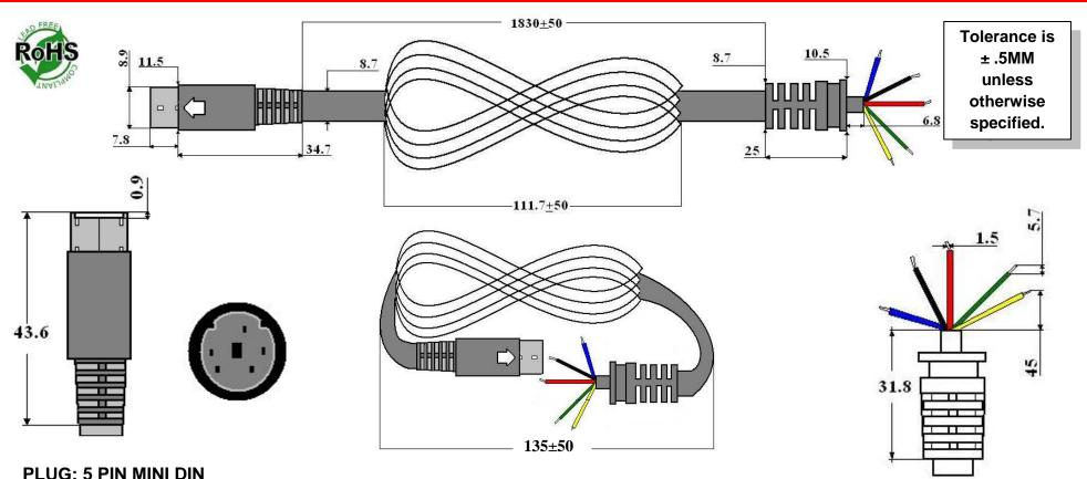
END: FIVE COLOR-CODED WIRES WITH STRIPPED AND TINNED LEADS AND A STRAIN RELIEF.
