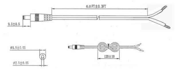
PLUG: 206 DETENTED WITH INSULATED TIP (2.5 x 5.5x 9.5mm),
