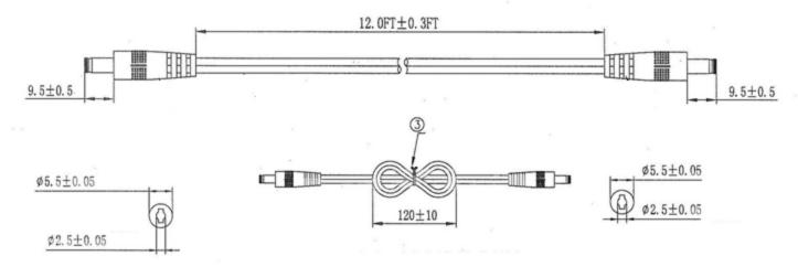
PLUG: 206 DETENTED WITH INSULATED TIP (2.5 x 5.5x 9.5mm),
