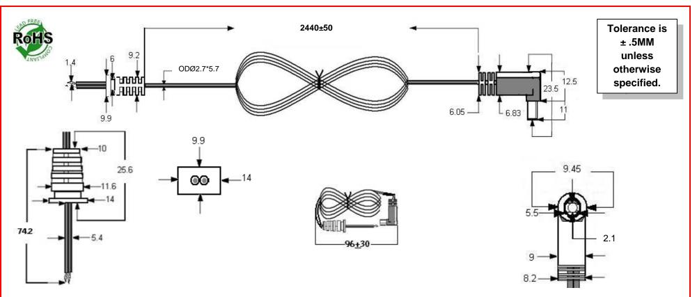
PLUG: 205(2.1 x 5.5 x 11mm) RIGHT ANGLE, WIRE WITH WORDING IS POSITIVE
