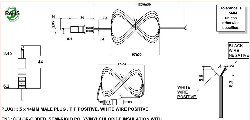
END: COLOR-CODED, SEMI-RIGID POLYVINYLCHLORIDE INSULATION WITH STRIPPED AND TINNED LEADS
