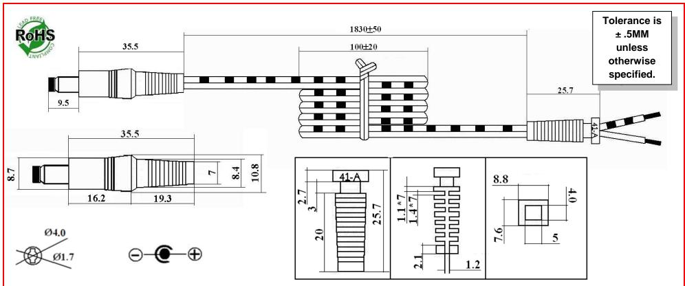
FIRST END: 1.7 x 4.0 x 9.5MM DETENTED FEMALE PLUG, WHITE WIRE POSITIVE
