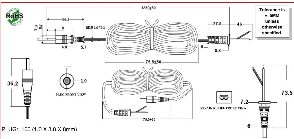
END: STRIPPED AND TINNED LEADS WITH STRAIN RELIEF
