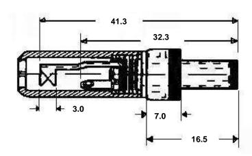
PART DC Locking Plug, 2.1 x 5.5 x 9mm, I.D. Hard Plastic
