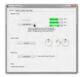
The last step in the calibration process is to set a "zero" or home position, your natural orientation when looking level and straight ahead while using the eyewear.
