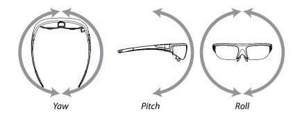
Continue to rotate the eyewear through all axes until all movement of the indicated progress bars cease. The indicator bars will not fill completely – this is normal.
