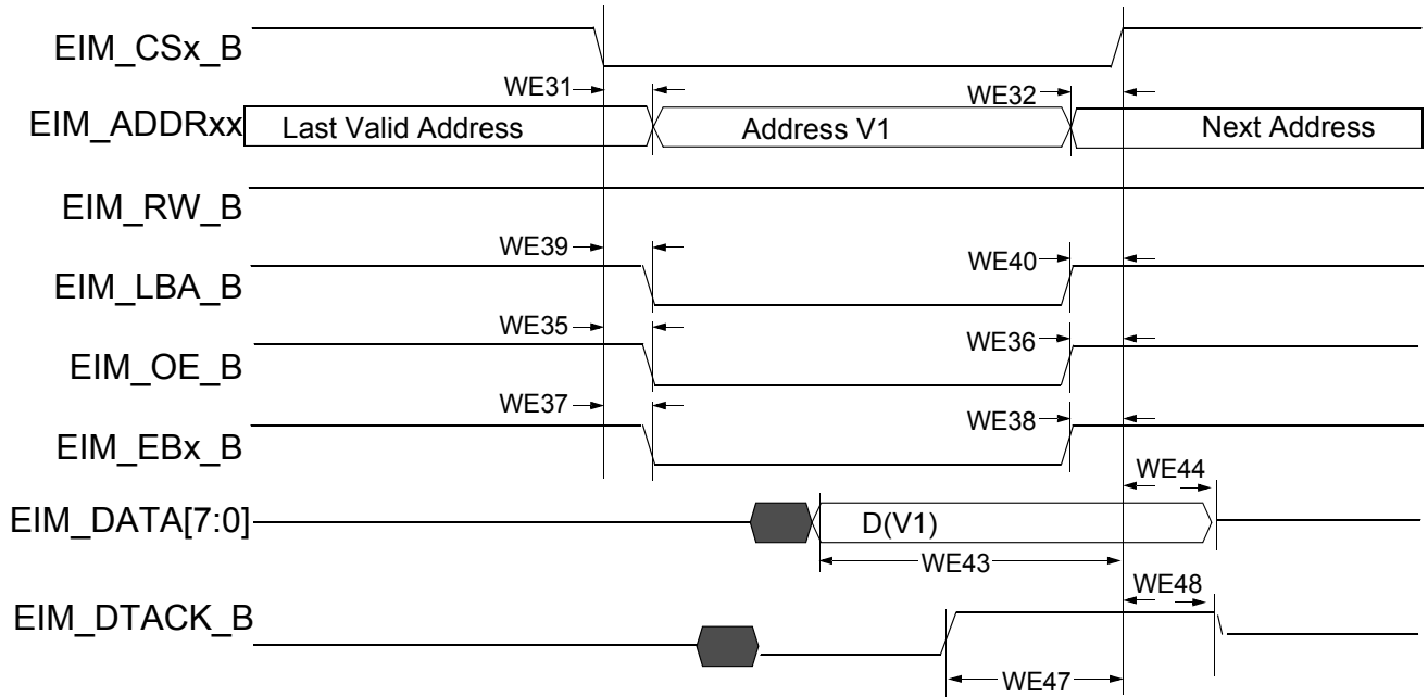
Figure 20. DTACK Read Access (DAP=0)
