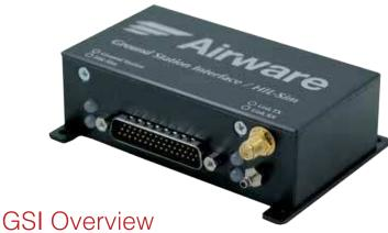
The Airware Ground Station Interface (GSI) with Hardware-Inthe-Loop Simulator (HIL-Sim) is a combination of autopilot command and control interface and rapid development/test platform for Unmanned Aerial Systems (UAS). It interfaces with AirwareOS autopilots for autonomous and manual control of vehicles in-flight and enables real-time simulation of missions and development of new capabilities on the ground.
