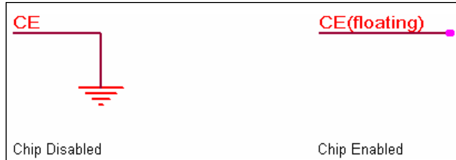
Figure 7-1 CE Pin Connection Option
