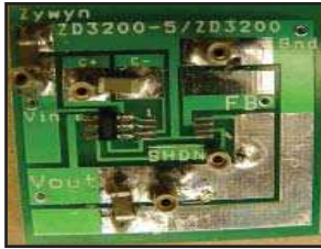
Figure 5. ZD3210EVB Evaluation Board Component Side Layout
