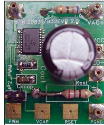
Figure 11. ZD832EVB Evaluation Board Component Side Topview
