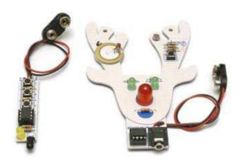
The Rudolf project PCB is supplied with a small optional 'infra-red' upgrade PCB. When populated with components, this infra-red PCB can be used to remotely control the Rudolf Cyberpet decoration. The components required are supplied in kit AXE-108K
