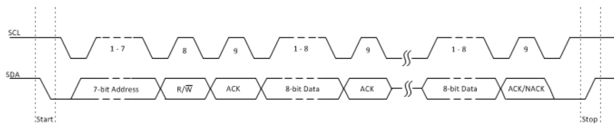
Figure 10-8: I2C Timing Diagram
