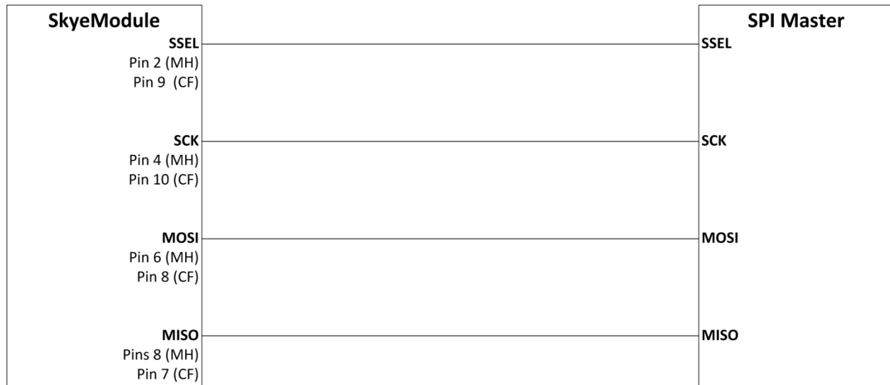
Figure 9-3: SPI Connection Diagram
