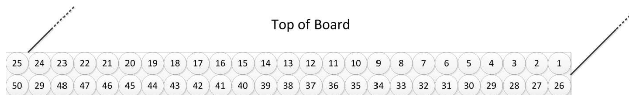
Figure 6-2: M2-CF Pin Numbering
