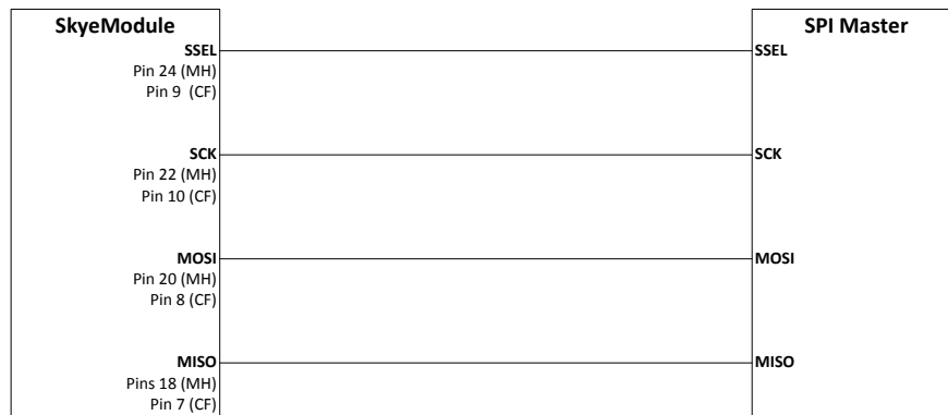
Figure 9-3 SPI Connection Diagram
