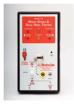
**Easy to use:** Position selector switch according to desired test: wrist, feet, or both simultaneously. Step on footplate then press and hold the button. The green "OK" LED will illuminate for a pass and one of the red LEDs will illuminate for a failure. A buzzer will also sound for failed tests. Red lights will signify whether an employee tested too high or too low, or whether there was a wrist strap failure or a heel grounder failure. Details of testing are found in the ACL 780 manual.
